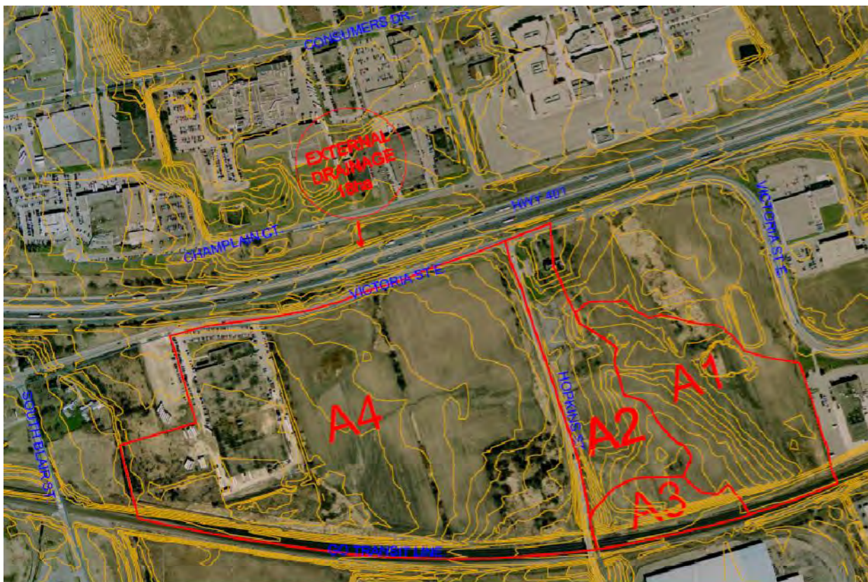
Figure 2.1. Existing Drainage Areas
