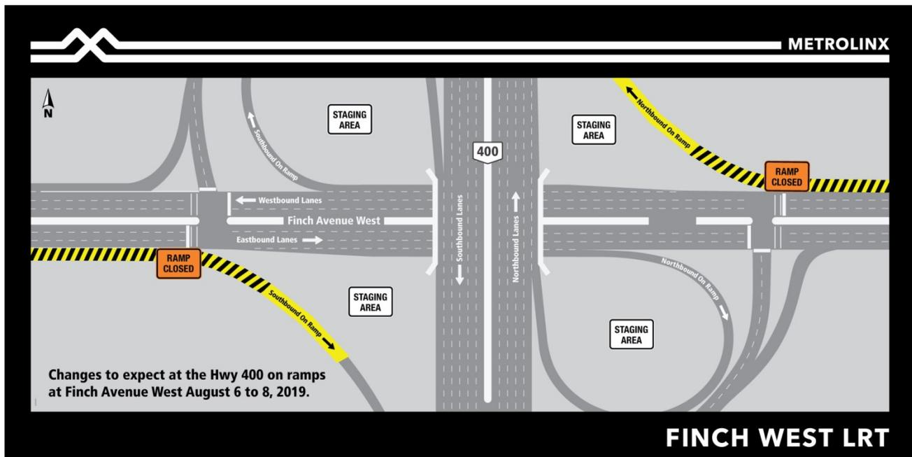
**Why:** Overnight closures of the on-ramps will take place to allow a crew to install the concrete barriers to protect workers and motorists during works to rehabilitate the Highway 400 bridge, which is included in the Finch West LRT project.
