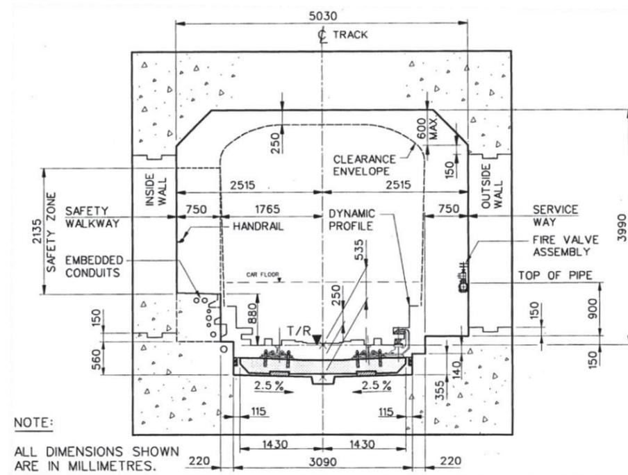
Exhibit 2: Typical Single Box Section – Double Tie, Tangent Track (Source: TTC DM-0205-01)
