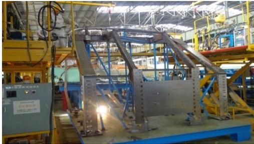
*Construction of front cab shell at Nippon Sharyo manufacturing plant*
