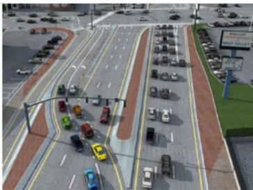
*Continuous Flow concept as applied in Salt Lake City (photo image: UDOT)*
