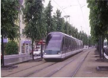
LRT making use of a broad arterial median right-of-way (Strasbourg, France). Photo: lightrailnow.org
