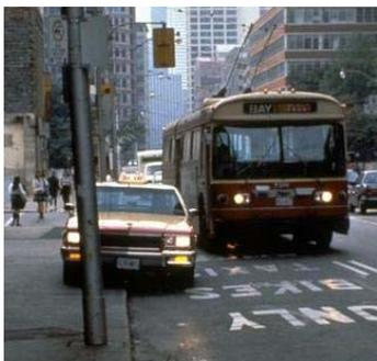
Different functions competing for use of the curb lane on Toronto's Bay Street; access restrictions need to be enforced to be effective on an arterial
